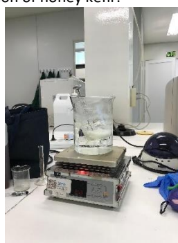
(b) Pasteurization for 15 Seconds at 72°C using the Double Broiler Method
