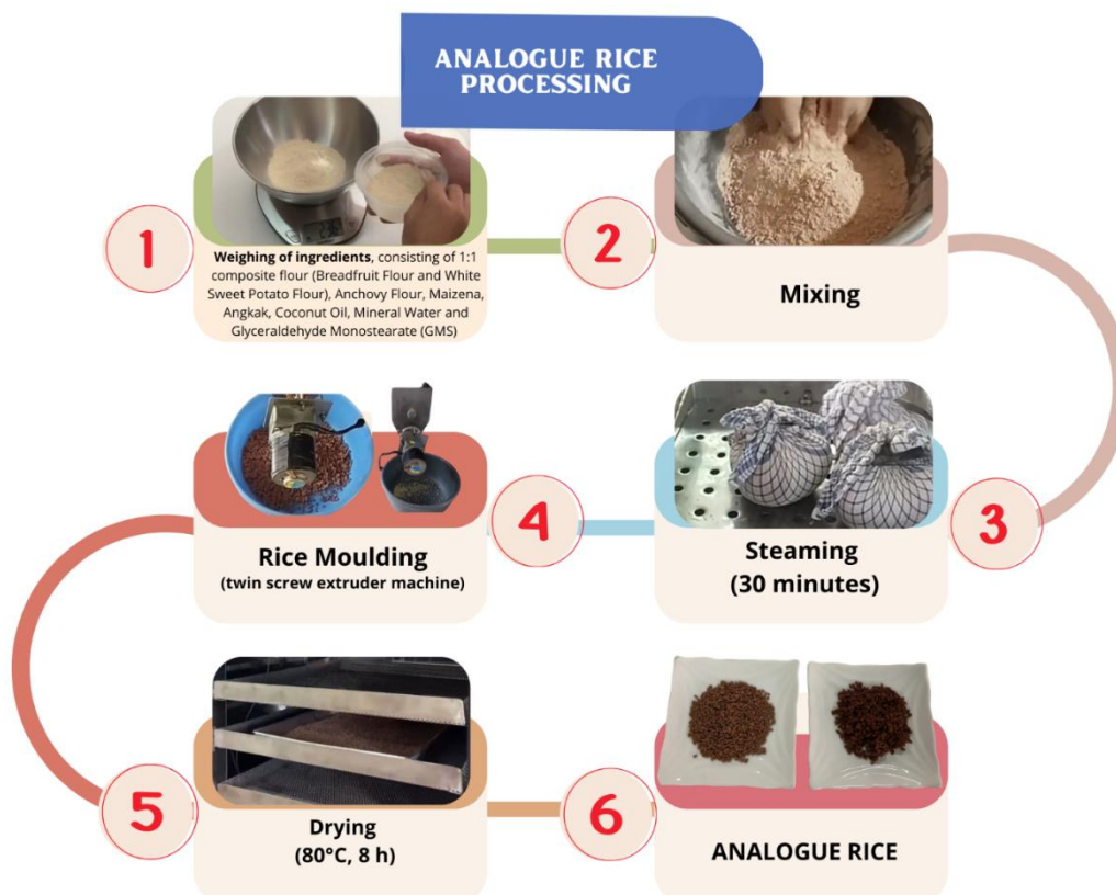
Figure 3. Flow Diag of Analogue Rice Processing Based on Breadfruit Flour ( Artocarpus Altilis ) and Anchovy ( Stolephorus Commersonii ) (Based on Modified by Zhang 29 , dan Santosa 20 )
