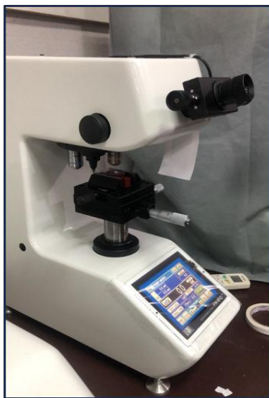
Figure 3. Microhardness test performed using a Vickers Microhardness Device (Future-Tech Corp, Japan).
