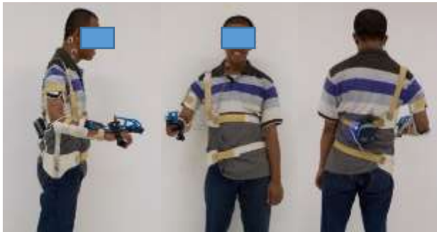
Figure 2. Myoelectric prehension orthosis installed on subject.
