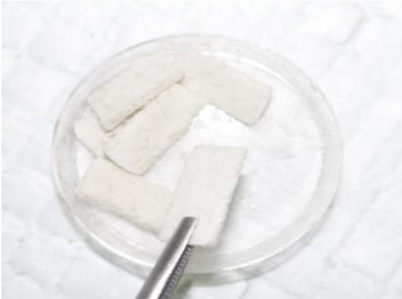
Figure 1. Macroscopic appearance of BCPRF implants showing porous compact texture
