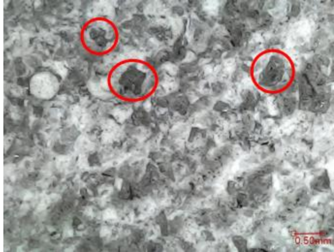
FIGURE 3. Results of macro observations of polymer concrete specimens with a weight fraction of 25% at 100X magnification
