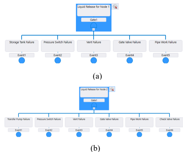
Figure 3. Fault Tree Analysis (FTA) Diagram for Liquid Release at a) Node 1 and b) Node 2
