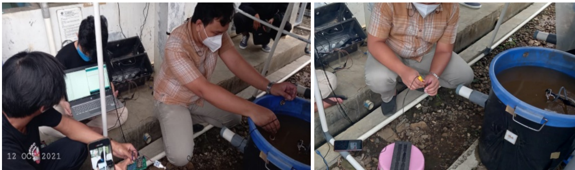
Figure 3. Display of the process of measuring oxygen levels in shrimp culture media.
