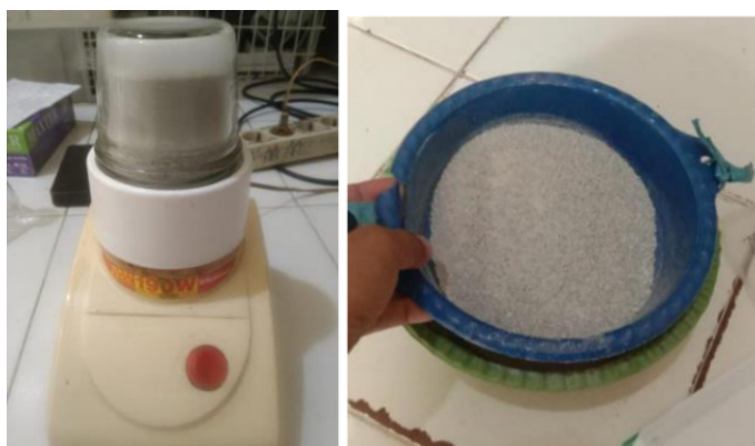
Figure 2. Processing of green mussel shells into shell powder.
