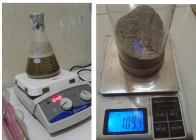
Figure 4. Nano chitosan was synthesized from chitosan using the ionic gelation method. Chitosan was first dissolved in a 10% acetic acid solution at a ratio of 1:10 (chitosan: acetic acid) to protonate the amino groups and enhance solubility. Then, 0.1% sodium tripolyphosphate (NaTPP) was added at a 7:1 ratio (chitosan solution: NaTPP). As a crosslinking agent, NaTPP facilitated ionic interactions between the positively charged chitosan and negatively charged phosphate groups, resulting in the formation of nano chitosan as a dispersed solid.
