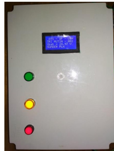
Figure 11 Front view of the panel when the battery voltage is 24.5-25.5 Volts with undervoltage conditions towards rating
