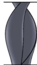
Figure 2. Helical bucket shape [18]
