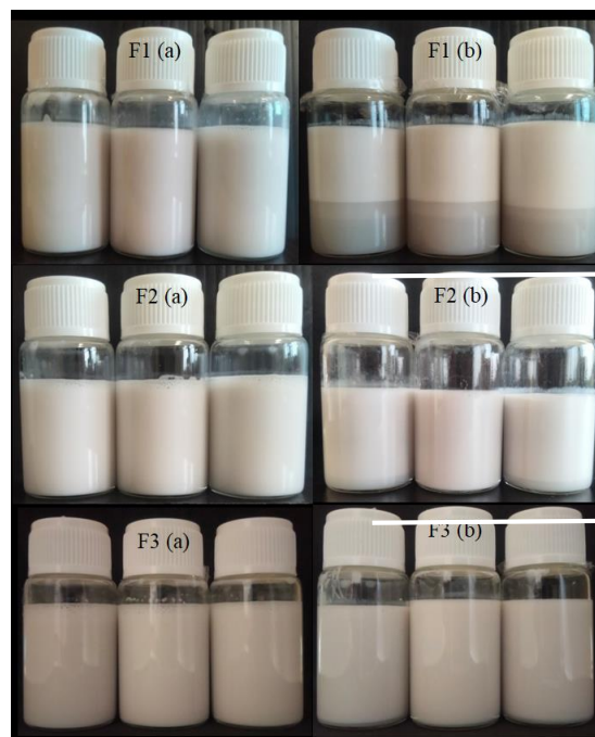
Figure 3. Physical stability test results of NLC-GTE [(a) before cycle; (b) after cycle]
