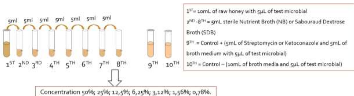
Figure 2. Serial dilution method with ratio 1:2 (v/v)
