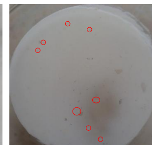
Figure 2. Homogeneity test results. Red circles indicate unmixed collagen hydrolysate granules
