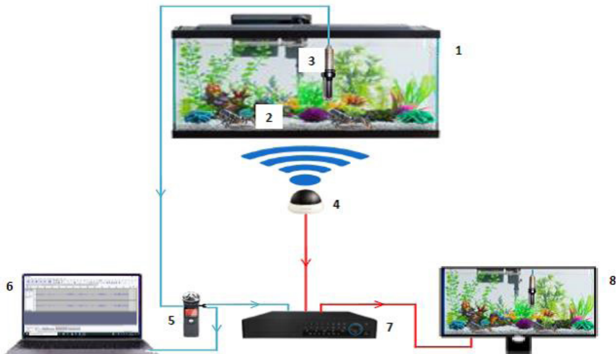
Figure 1. Recording systems. The blue and red lines represent the audio and video line (1–8) represented aquarium, lobster, hydrophone, CCTV camera, sound recorder, personal computer, video recorder, and LCD monitor, respectively
