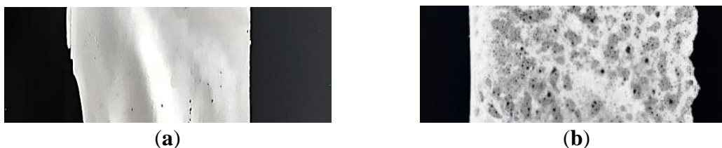
Figure 2. Images of polystyrene (PS) membranes from Styrofoam waste prepared by (a) immersion and (b) evaporation treatment.
