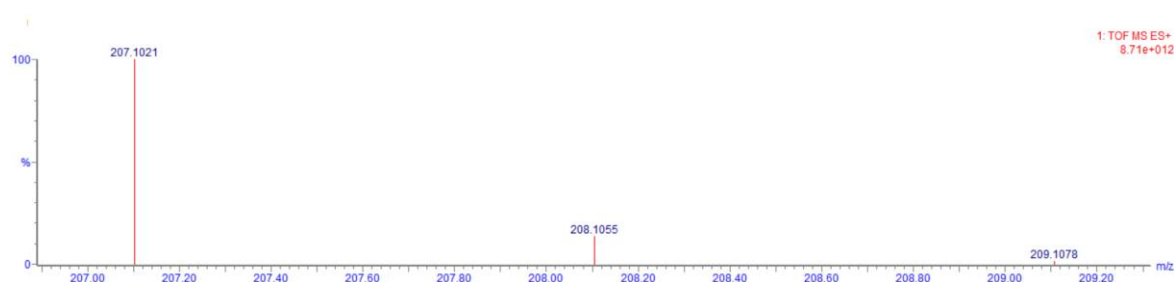
Figure 8. Mass spectra of ethyl trans- p -methoxycinnamate
