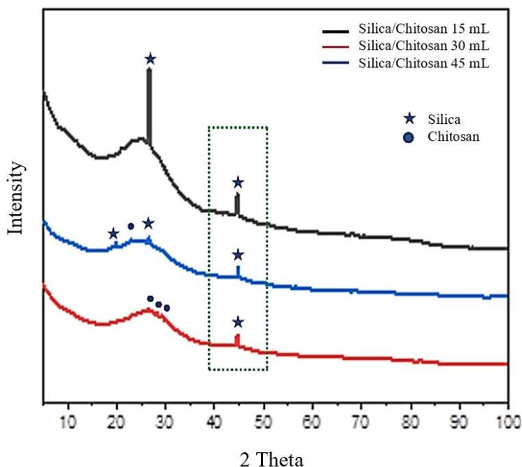
**Figure 2.** Diffractogram of silica-chitosan
