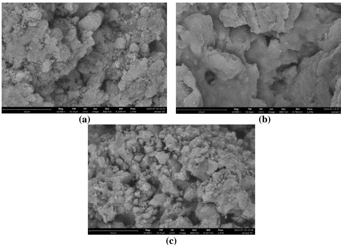
**Figure 4.** SEM analysis results of silica chitosan composites (a) 15 mL (b) 30 mL (c) 45 mL at 10,000× magnification.
