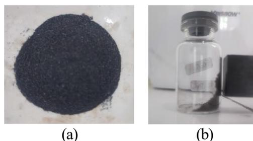
**Figure 1.** (a)  $\text{Fe}_3\text{O}_4$  material, (b) magnetic properties test to an external magnetic field
