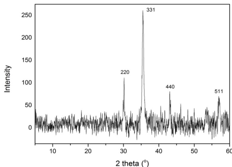
**Figure 3.** XRD diffractograms of  $\text{Fe}_3\text{O}_4$
