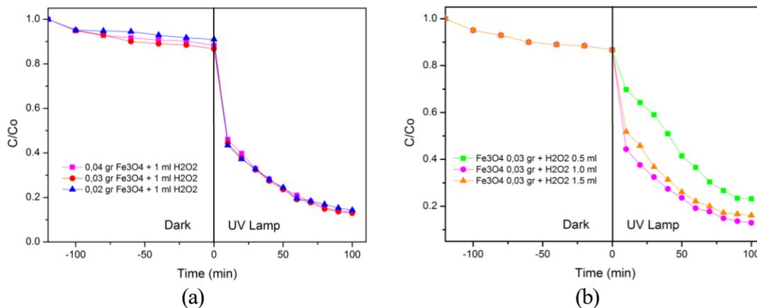
**Figure 4.** Photo-Fenton degradation of HA activity curves with different weights of (a)  $\text{Fe}_3\text{O}_4$  catalyst, (b) volume of  $\text{H}_2\text{O}_2$
