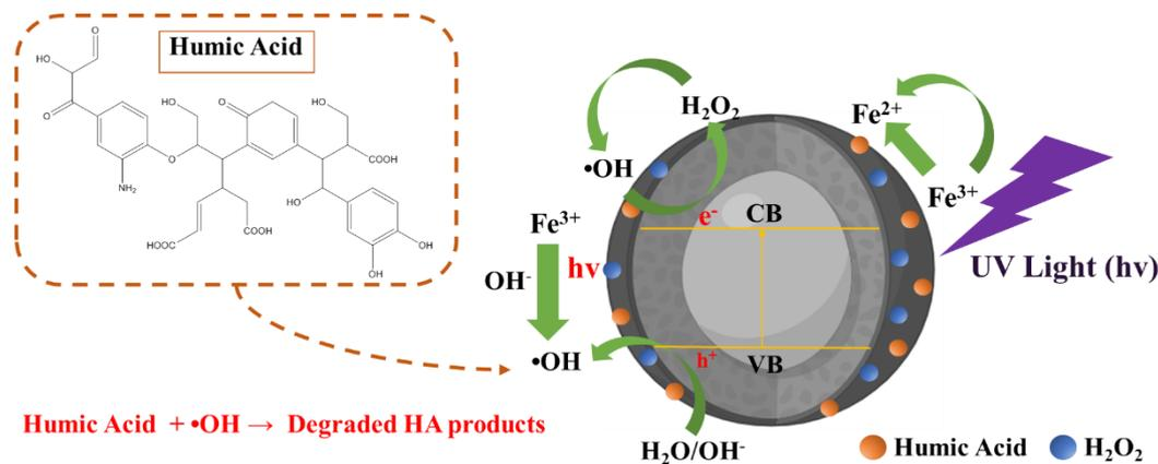
**Figure 6.** Cycle of Humic Acid Degradation via Fe<sub>3</sub>O<sub>4</sub> Fenton Catalyst
