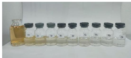
**Figure 5.** Photo-Fenton degradation activity curves of HA with different condition (a); and colour change of HA degradation (b)
