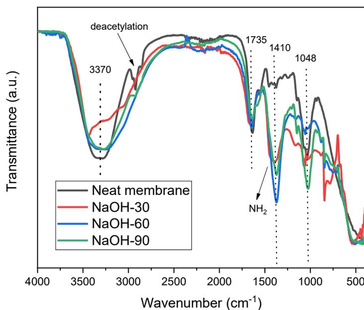
**Figure 2.** FTIR spectra of hydroxylated-fungal-derived membranes
