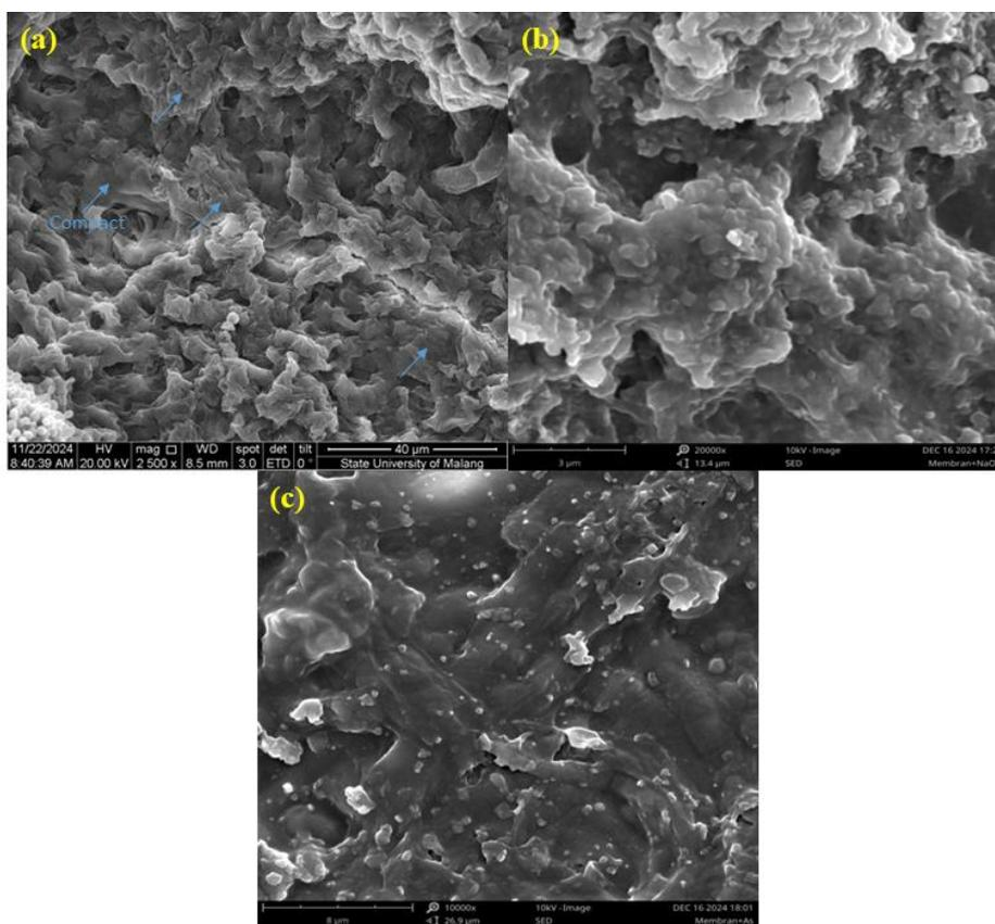
**Figure 4.** SEM photographs of the unmodified fungal-derived membrane (a), hydroxylated fungal-derived membrane (b), and stearic acid-coated fungal-derived membrane (c)
