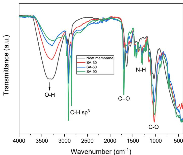
**Figure 3.** FTIR spectra of stearic acid-coated fungal-derived membranes
