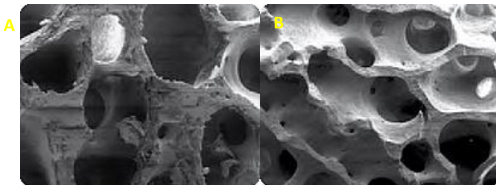
Figure 2. Microscopic structure of human human and bovine cancellous bone . Scanning electron microscope shows similarity in architecture and bony porosities between human cancellous bone (A) and bovine cancellous bone (B) (Fassina et al., 2010)
