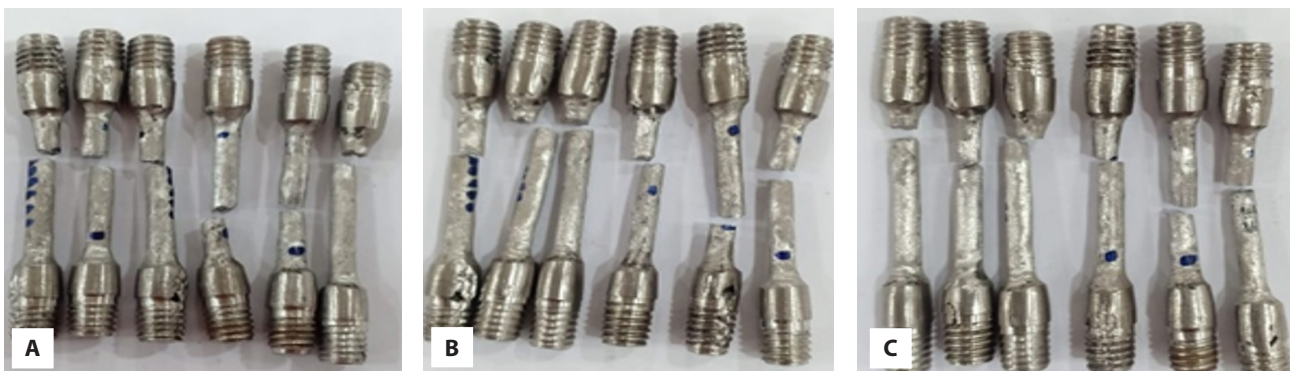
Figure 3. Results after tensile test to break. (A) New 100% CoCr metal, (B) New 50% CoCr metal + 50% repeated, (C) 100% repeated CoCr Metal
