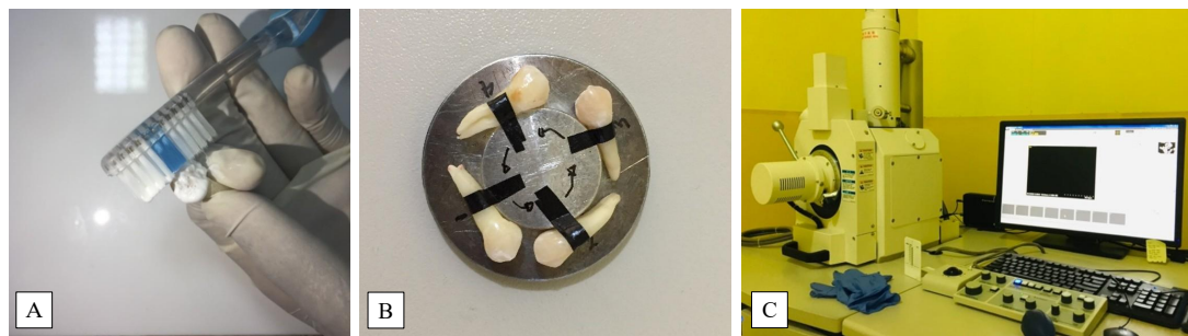
Figure 3. The application of the material and the analysis processes. A. Novamin application on groups III and V, B. SEM observation, C. The application of SEM with energy-dispersive x-ray spectroscopy (EDX) analysis.
