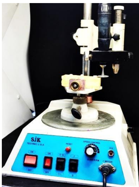
Figure 1. A milling machine is used to cut the ridge lap part of synthetic teeth.
