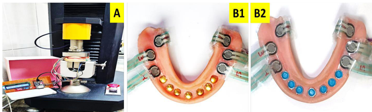
Figure 3. Retention test: universal testing machine (A) and channel sensors (B1 and B2).
