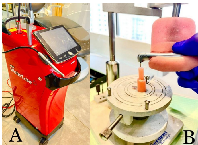
Figure 3. (A) Laser unit machine Er,Cr:YSGG (Water-lase, BIOLASE). (B) Application of laser on an acrylic surface.
