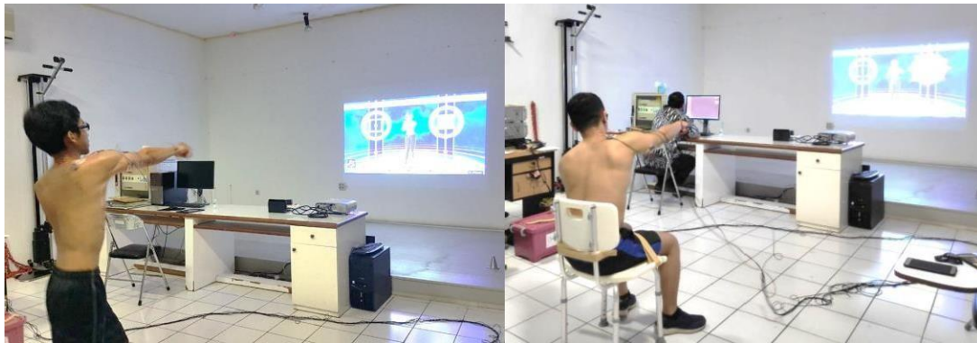
Figure 1. Participants delivering straight punches while playing “Fitness Boxing” using Nintendo Switch™ with electrode attached on four upper limb muscles in standing and sitting position
